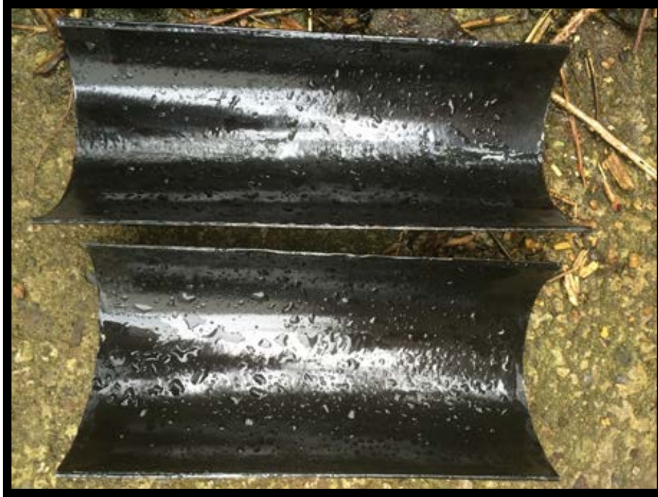
PX painted Gutter
