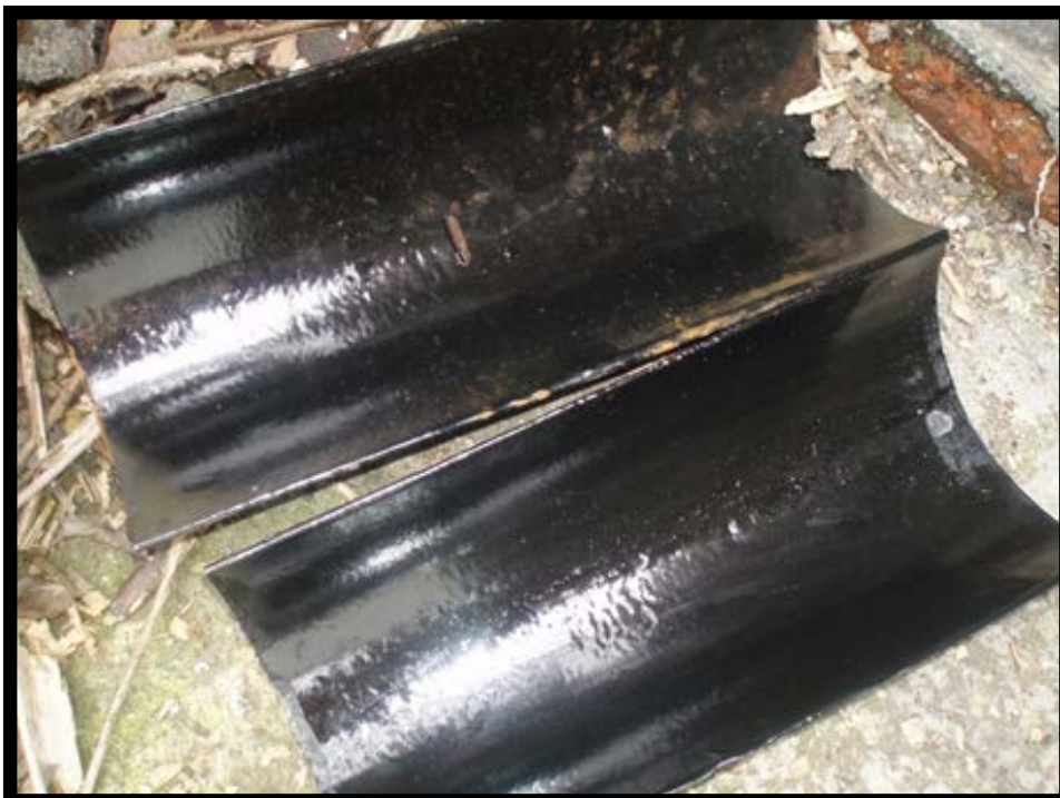
PX painted Gutter -
