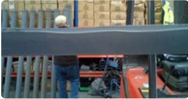
Examples of poor quality, warped gutters
