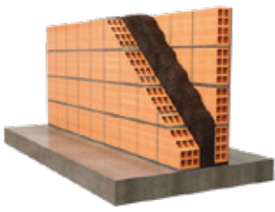
Internal partitions Filling the internal double walls with expanded cork granules
