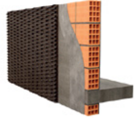
External walls Exterior cladding - cork at sight wave facade s1
