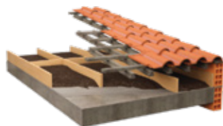
Roofs Pitched roof with loose fill insulation between joists
