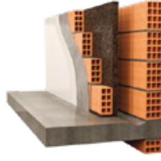
External walls Exterior cladding with shiplap system - cork at sight
