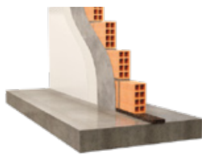
Internal partitions Masonry wall and slab discontinuity
