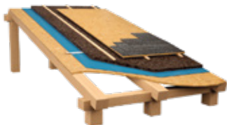
Roofs Pitched roof with above rafter insulation
