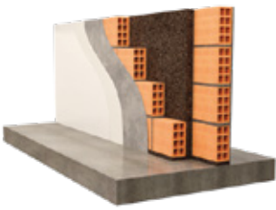
Internal partitions Double wall with insulation fully filling the cavity
