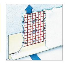
Ventilation gaps located at both top and bottom of the system allow circulation for this purpose.
