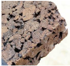
SecilVit Cork board Available 500 x 1000mm in either 40,60,80,100mm thickness. K value = 0.036-0.040 w/mk
